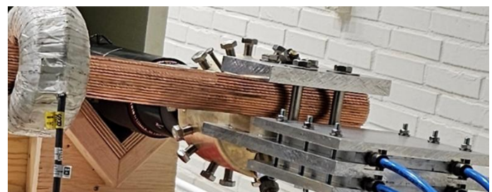
Laminated Cu used to reduce losses
